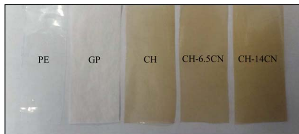
Figure 4. The visual appearance of PE, GP, pure chitosan, CH-6.5CN, and CH-14CN films. [Color figure can be viewed in the online issue, which is available at wileyonlinelibrary.com .]
